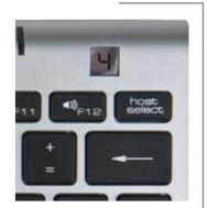
When pairing multiple devices to the M-board 870 Bluetooth Keyboard, press the host select key (D) and select the device number using number keys 1-8 (A). The mini-display window (C) indicates the active device.
