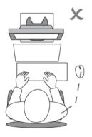
Compact keyboard M-board 870, reduces the distance a user has to reach for operating the mouse and allows a more comfortable body posture.
