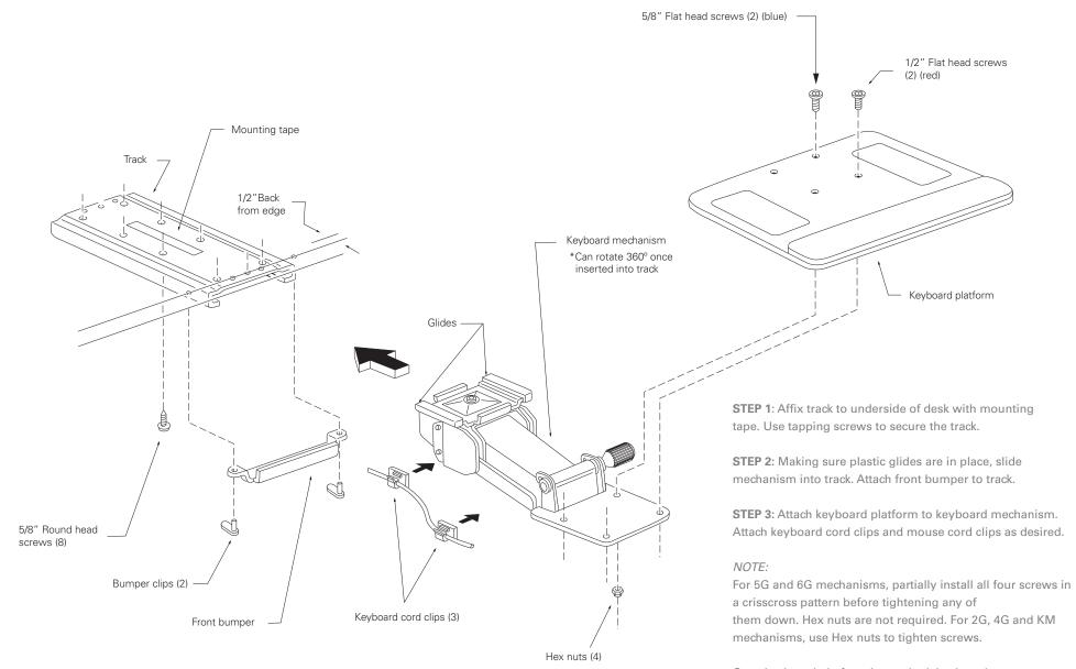
Once keyboard platform is attached, keyboard system can be lowered and raised as needed, and will stay firm in desired position.
