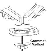
**2.** Peel the adhesive backing from the clamp pad and attach the pad to the base and grommet mount plate.
